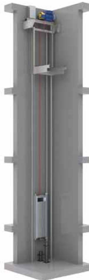
Cantilevered elevator in suspension 1:1
